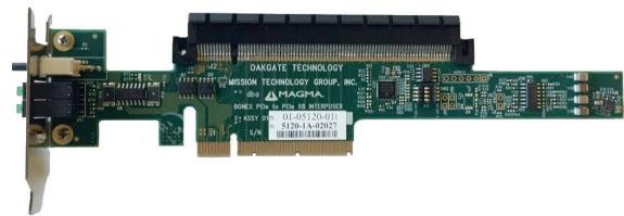
Figure 1. PCIe Power Interposer Card for OakGate Appliances and 7-Slot PCIe Enclosure (OGT-AP100)
