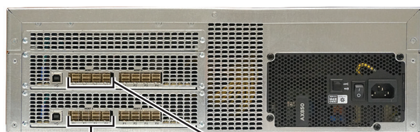
Bottom P1-P4 SFF-8644 Connectors for Single Port or Dual-Port NVMe SSDs Top P1-P4 SFF-8644 Connectors for Dual-Port NVMe SSDs
